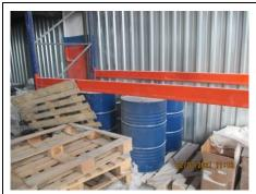
NC#2: There are no secondary containers for the solvent barrels in the production area.
